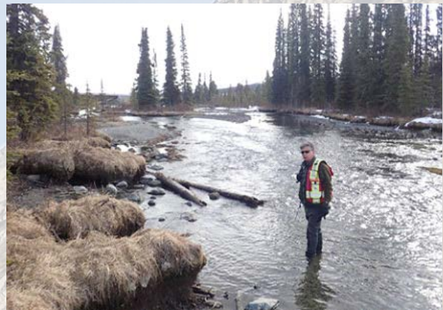
Image shows 0.8 m 3 /s flow in Upper Pine Creek, which is HALF of what would be expected
